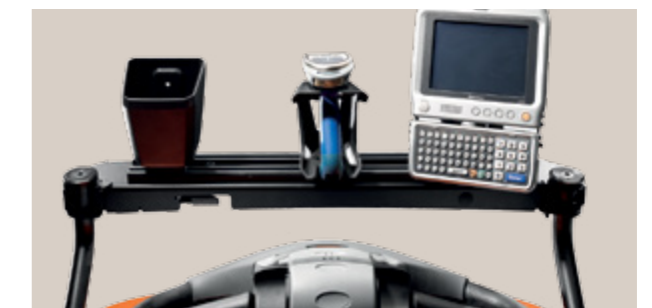
The BT Movit S-series E-bar option allows the mounting and powering of ancillary equipment such as computers and barcode scanners.
