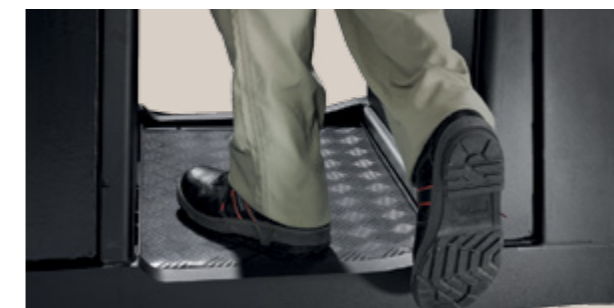
The TSE300's low step-in height reduces the strain of repeatedly stepping into and out of the truck. The floor is suspended to reduce vibration, enhancing driver comfort.
